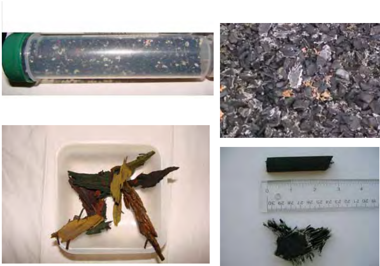
Figures 5 through 8. Tire crumb infill granules from site F2 (top left), shredded tire crumb at site P1 (top and bottom right), and tire crumb material from site P2 (bottom left).
